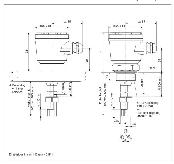
Dimensions of the three-rod probes 11363 and 11363 Z. Height and diameter are similar for all housings.
