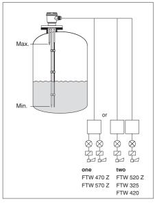
Detection of a minimum and maximum level limit in a plastic vessel
