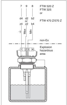
Two-point control in a plastic vessel without cable monitoring and also for use in explosion hazardous areas
