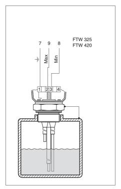
Two-point control in a plastic vessel without cable monitoring
