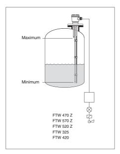
Two-point control in a plastic vessel
